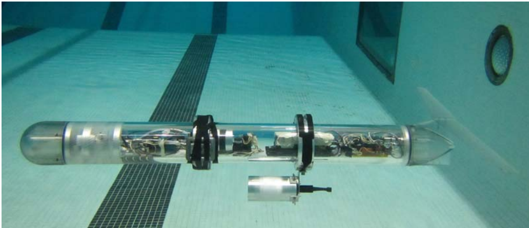
Figure 2.4: An ECO-Puck chlorophyll-a sensor in aluminum casing attached to the ROUGHIE's exterior. It connects to the internal electrical system via a waterproof cable through the rear end cap (not shown in this image).
